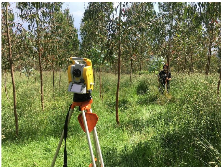
Figura 2. Eucalyptus geo-positioning in the field using a total station
