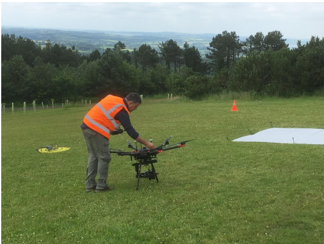
Figure 9: Preparing a drone with a thermal camera for a flight during the field training session in JFK Arboretum
